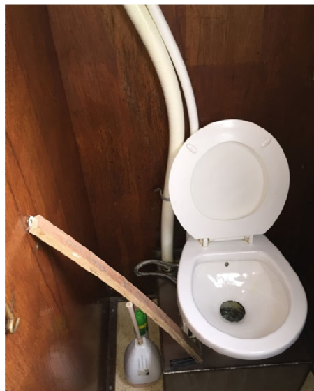
Front loo, foot pedal jammed open.
